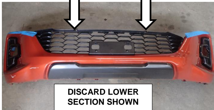
Unclip from upper section of bumper
